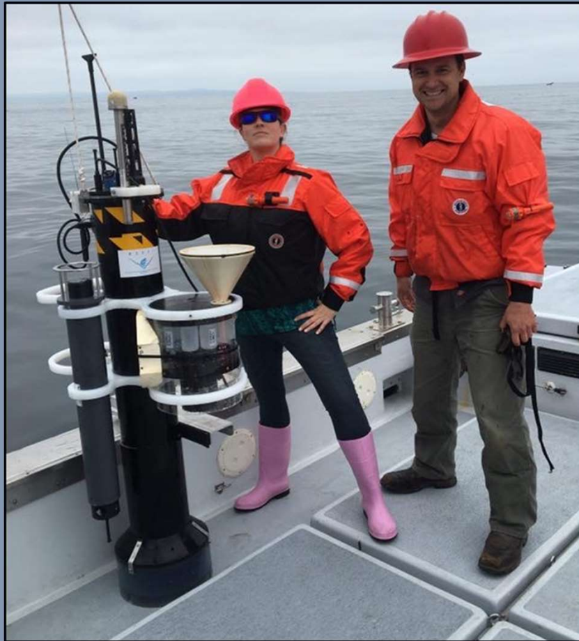
CPF V1.1 with sediment trap and acoustic modem
