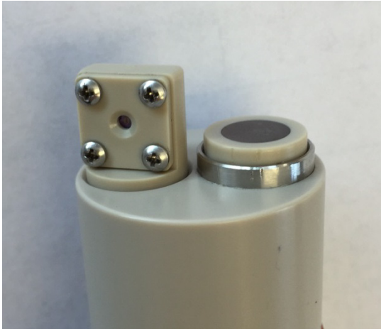
Fig. 2. ISFET, center of probe on left. Counter electrode, ring around probe on right. ISE, dark top part of probe on left.
