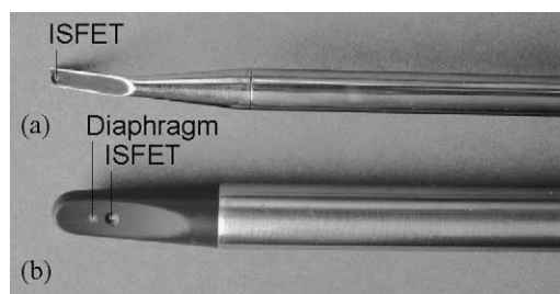
Fig. 7. Examples of ISFET sensors for special medical applications: (a) probe for measurements in dentistry, (b) probe for measurements in gynaecology.
