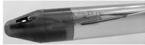
Fig. 13. Photograph of the tip of a Sentron ConeFET probe.
