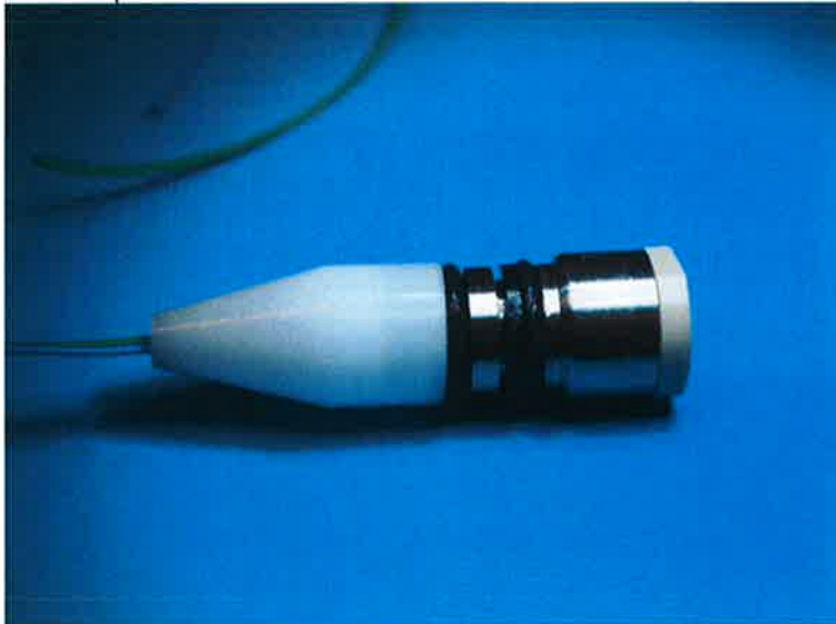
Figure 19: O-Rings Installed on Electrode
