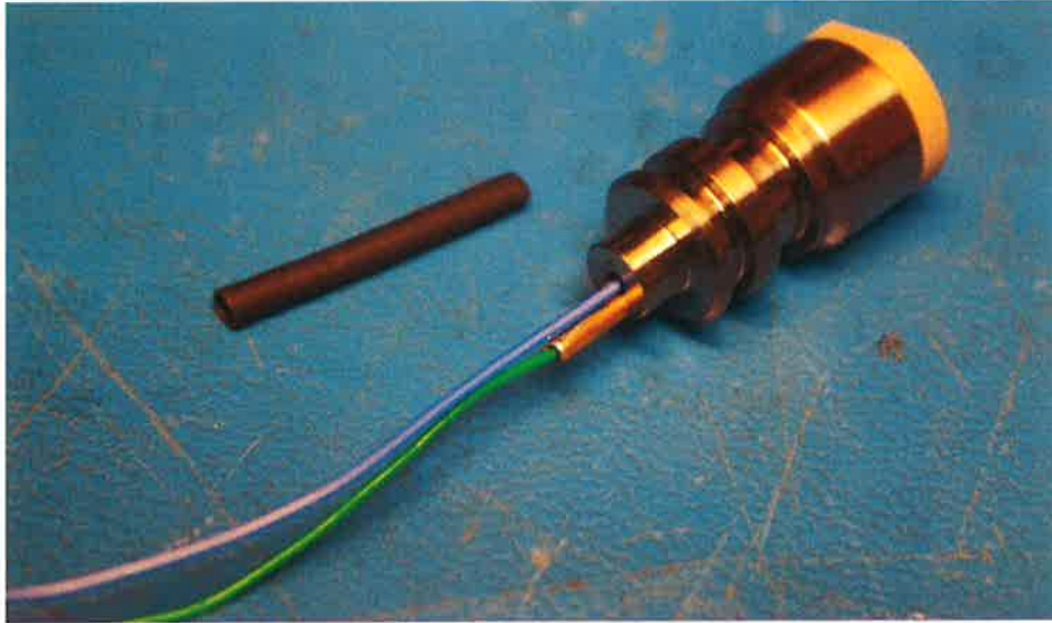
Figure 16: Reference Electrode place in Counter Electrode
