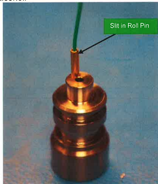
Figure 14: Counter Electrode with Soldered Wire
