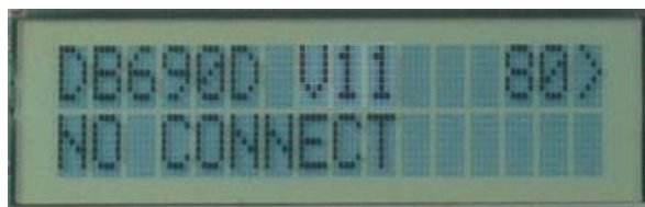
Figure 2: Startup with no encoder attached
