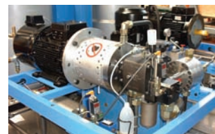
Maintenance-free sealing of dosing pump for polyde and isocyanate in high-pressure reaction casting machines
