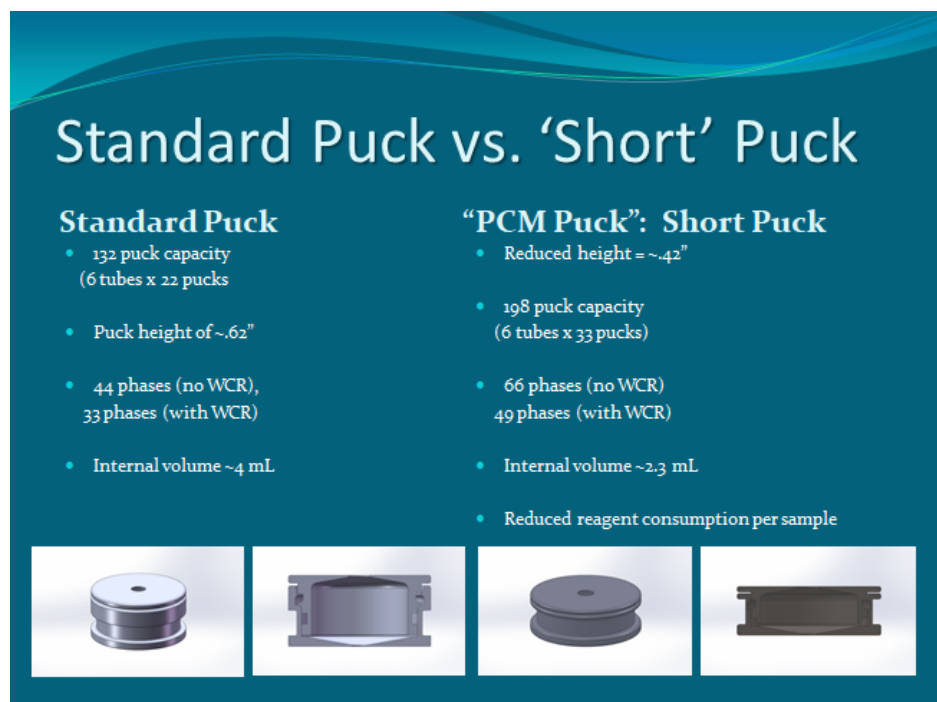
Figure 1: Comparison of Standard Puck vs. Short Puck
