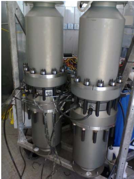
Fig. 3 DWSM assembly with flanges and jacket bolts for 20 MPa pressure validation prior to deployment. The jacket bolts are pre-tensioned to maintain seal integrity when internally pressurized.
