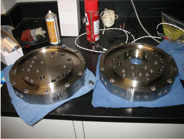
Fig. 2 Sample and Exhaust bulkhead plates for 4000m DWSM, made from 6Al4V titanium, Exhaust plate on right. Over 100 hours of CNC machining was required, and helical mill threading was used for the 80 threaded holes.
