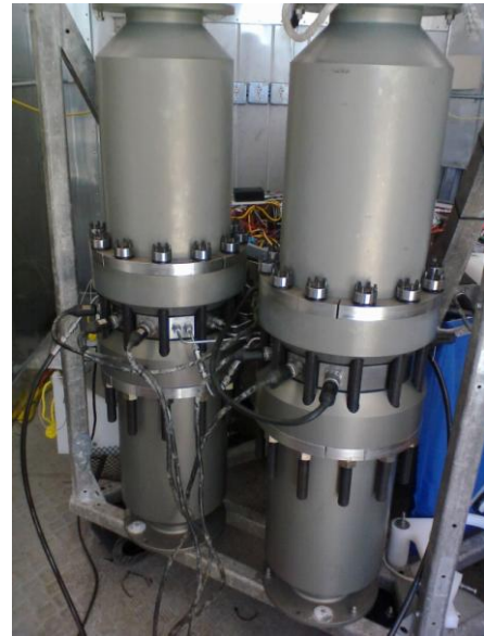
Fig. 5 DWSM assembly with flanges and jacket bolts for 20 MPa pressure validation prior to deployment. The jacket bolts are pre-tensioned to maintain seal integrity when internally pressurized.
