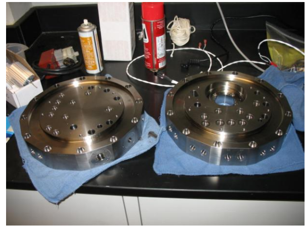
Fig. 4 Sample and Exhaust bulkhead plates for 4000m DWSM, made from 6Al4V titanium, Exhaust plate on right. Over 100 hours of CNC machining was required, and helical mill threading was used for the 80 threaded holes.
