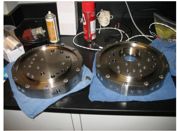
Fig. 3 Sample and Exhaust bulkhead plates for 4000m DWSM, made from 6Al4V titanium, Exhaust plate on right. Over 100 hours of CNC machining was required, and helical mill threading was used for the 80 threaded holes.
