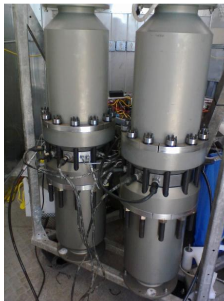
Fig. 4 DWSM assembly with flanges and jacket bolts for 20 MPa pressure validation prior to deployment. The jacket bolts are pre-tensioned to maintain seal integrity when internally pressurized.
