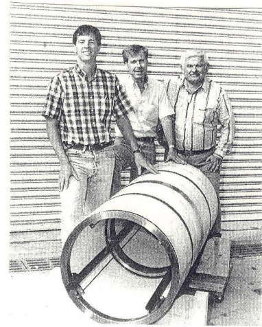
Figure 7 25 in OD X 64 in L ceramic housing for 20,000 ft depth service
