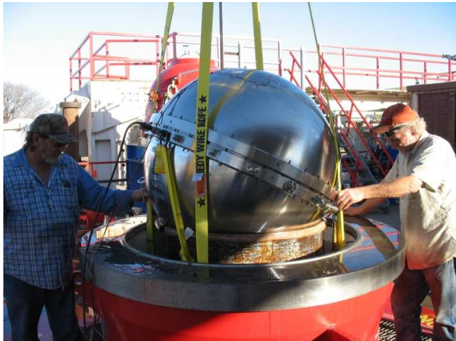
Fig. 8. Sphere being removed from hyperbaric chamber at SwRI after pressure testing to 41.4 MPa.
