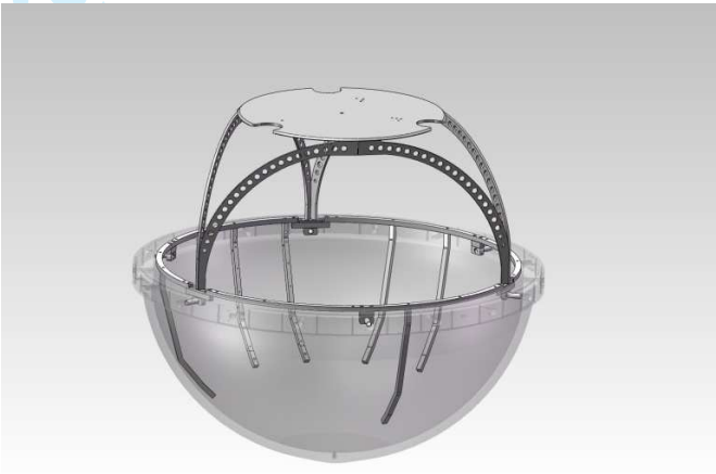
Fig. 11. Strain isolated internal mounting structure.
