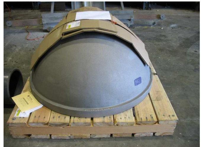
Fig. 4. Cast Ti-6Al-4V hemisphere, weighing 250 kg.
