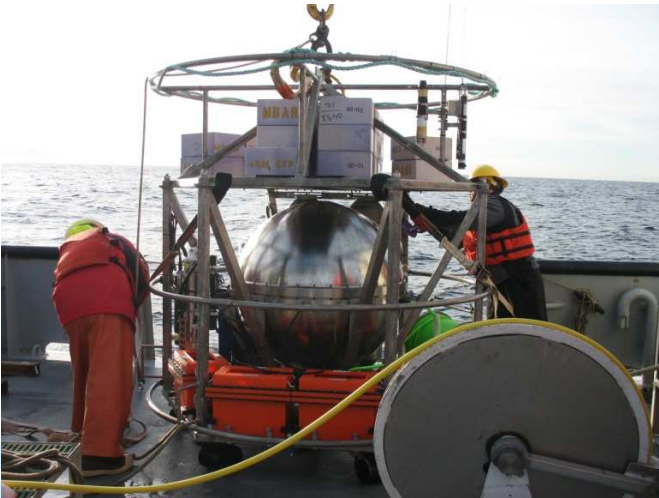
Fig. 10. The sphere, mounted in freefall elevator, is readied for deployment in the Monterey Canyon.
