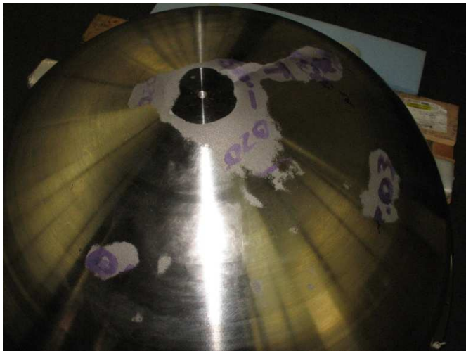
Fig. 6. Residual cast surfaces on top hemisphere.
