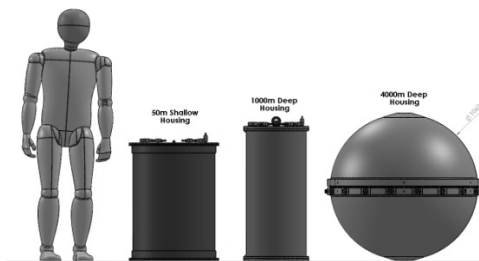
Fig. 1. Size comparison of ESP pressure housings.
