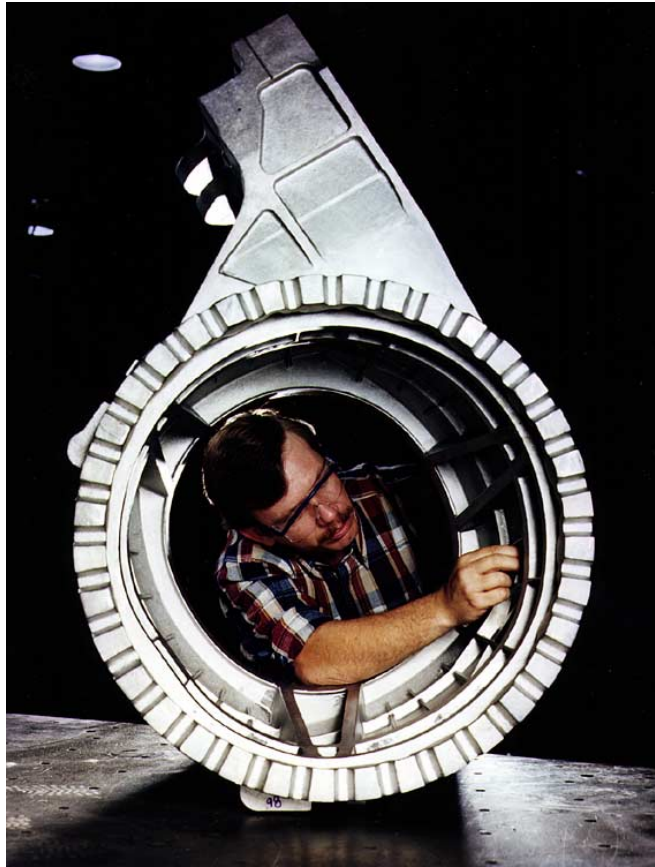
Figure 4. Investment Cast Bell Helicopter Transmission Adapter.
