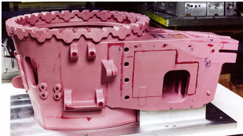
Figure 3. Bell Helicopter Transmission Adapter CAPM Pattern.
