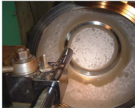
Machining the inside of a Ti 6-4 casting (above left) at the Monterey Bay Aquarium Research Institute. MBARI will join the machined dome with a sister half using compatible titanium hardware to create a water-tight, corrosion resistant sphere (below center) that houses very sensitive (and very expensive) seismological instrumentation (above right).
