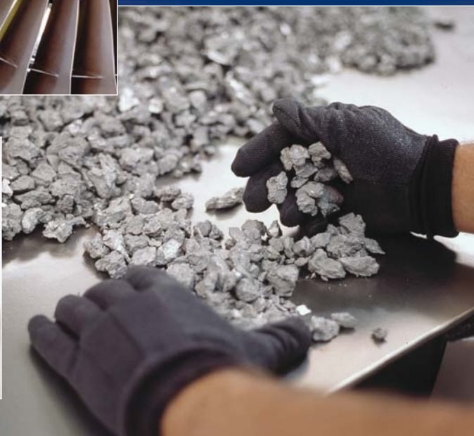
Titanium sponge is used in alloys for jet engine turbines (above left) and ultra light custom wheelchairs (bottom left).
