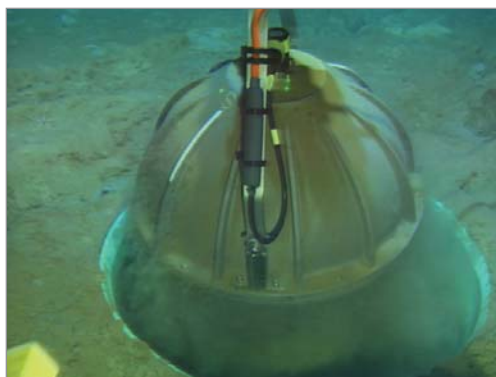
An ROV (Remotely Operated Vehicle) carefully positions a titanium sphere in a hole carved into the Pacific Ocean floor, over a mile below the surface.
