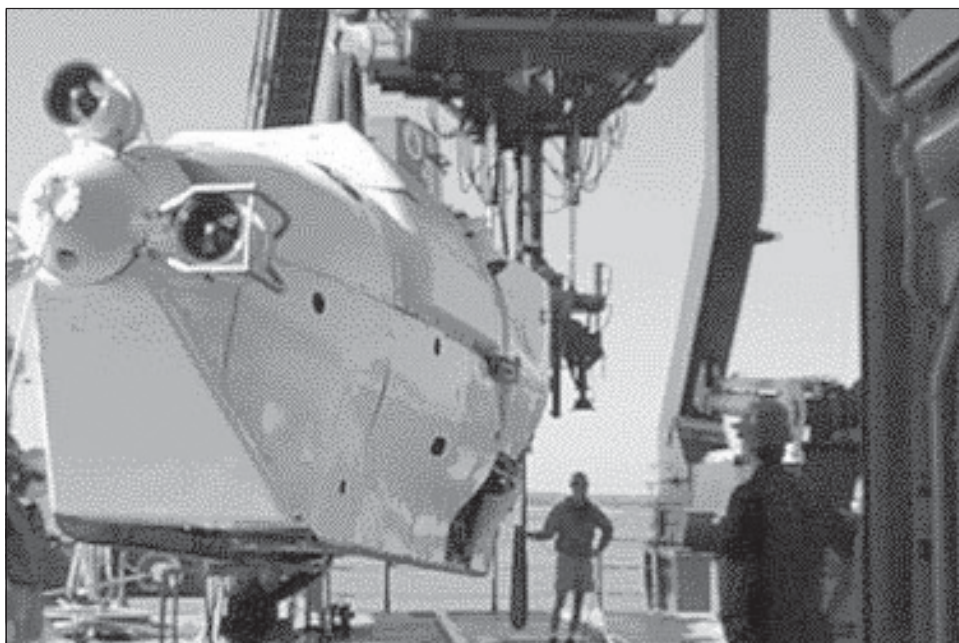
The new HOV must be compatible with the existing launch systems and storage hanger size on the Alvin 's research vessel Atlantis.
