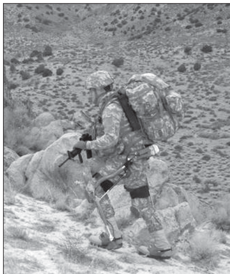
The Human Universal Load Carrier is a titanium exoskeleton that is attached to the outside of a soldier's leg, transferring the weight from heavy loads to the ground.
