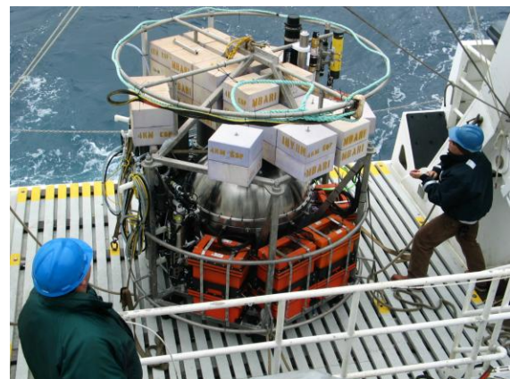
Fig. 1. D-ESP lander just before deployment. Titanium sphere houses the ESP instrument. In this view, DWSM is on the opposite side of the sphere.
