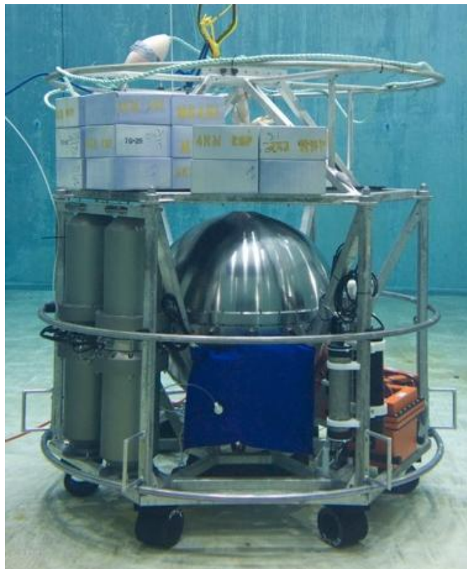
Fig. 3. Deep-ESP lander being tested in seawater tank prior to deployment. The titanium sphere in the center houses the ESP instrument. The green towers are the DWSM. The blue bag is the ambient oil reservoir. The orange boxes are batteries, and syntactic foam blocks are on the top.
