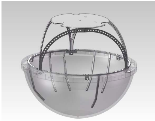
Fig. 10. Strain isolated internal mounting structure provides rigid support, allowing only concentric motion on the sphere.
