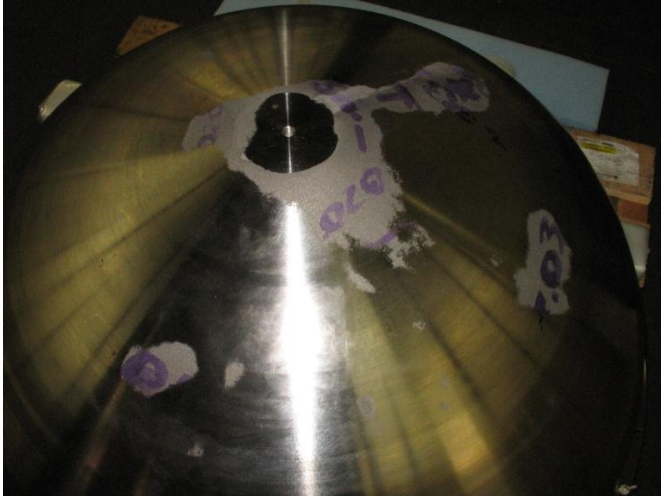
Fig. 6. Residual cast surfaces on top hemisphere after machining indicate localized thin spots on the shell. Additional FEA would determine that the stress concentrations would still be within our design factors.
