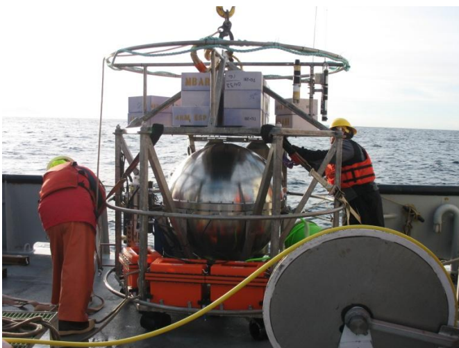
Fig. 11. The 1 m sphere, mounted in a freefall benthic lander sits on the deck of the R/V Point Lobos, and is being readied for deployment in the Monterey Canyon.
