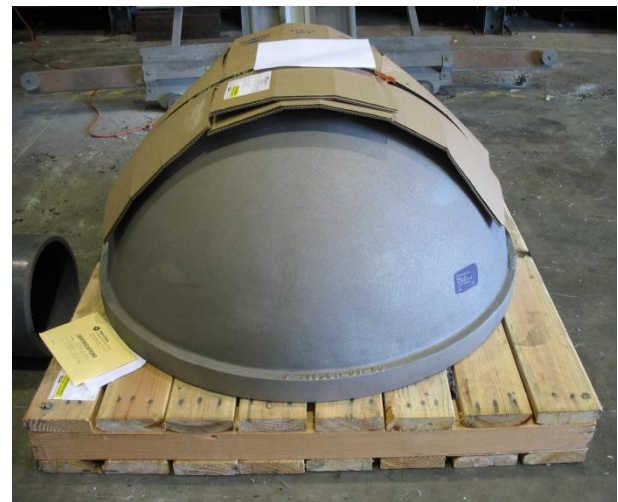
Fig. 4. Ti-6Al-4V near net shape cast hemisphere, weighing 250 kg. Such castings are poured in a rammed graphite mold, produced from hardwood patterns. The time to produce the patterns, make molds and pour the castings can exceed a year.
