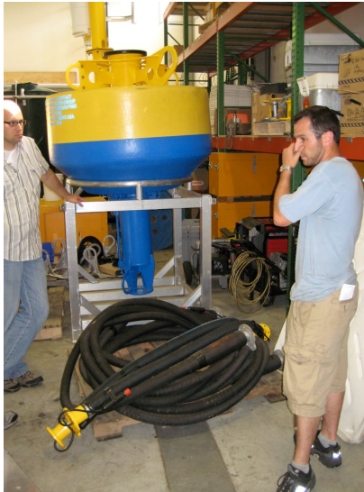
Short connectors b/w ESP and sphere
