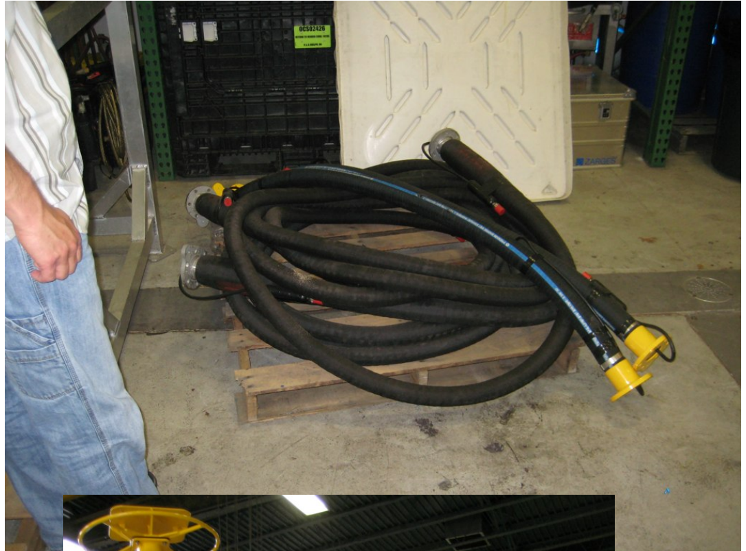
Long snubbers connecting sphere with mooring
