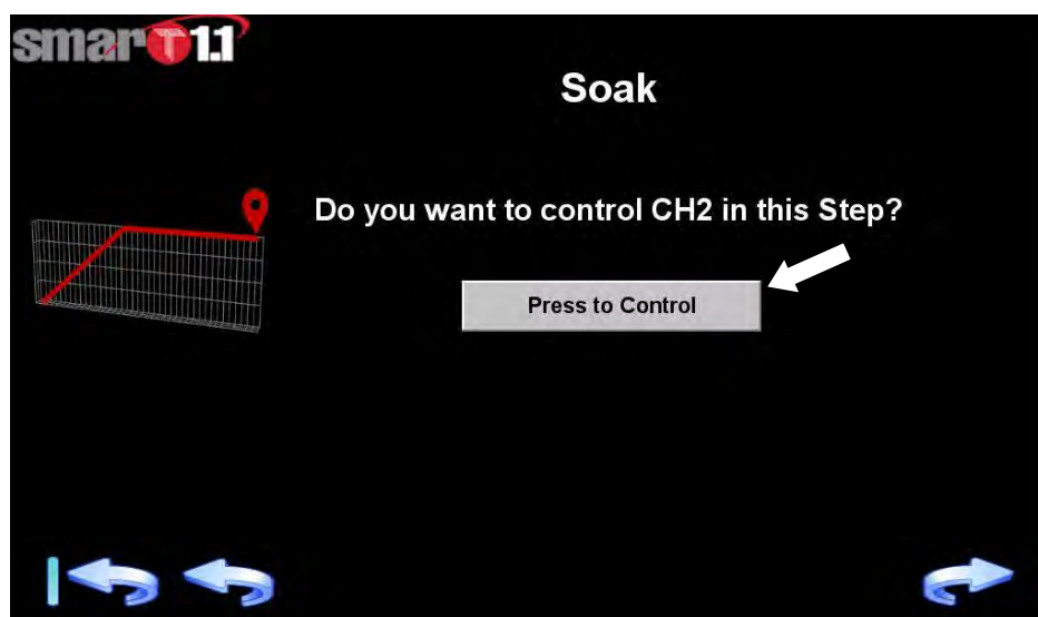
SOAK SCREEN – PRESS TO CONTROL CHAN. 2 SOAK HUMIDITY
