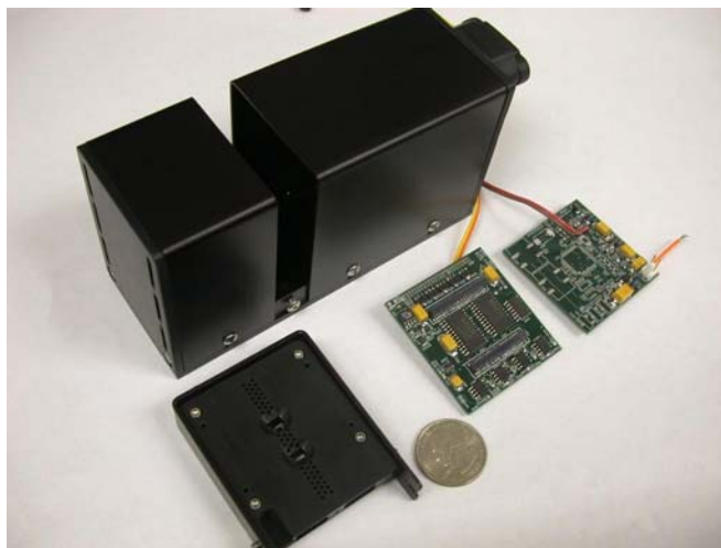
Figure 1. Some of the major components of the prototype ESP flow-through PCR module in assembly 2/28/2007: heater module (bottom left), analog board, digital board, and enclosure. The quarter will not be included in the production module.
