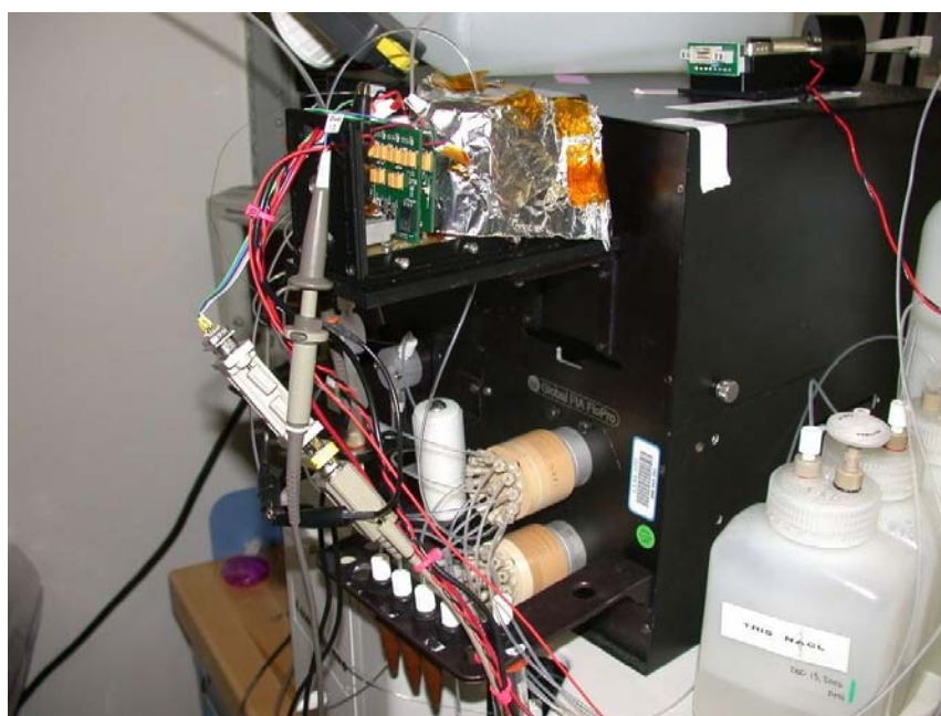
Figure 1. ESP flow-through PCR module integrated with an APDS-style (modified Global Flo-Pro) fluidics workstation. We had to fly some power lines in to the electronics boards and block light with foil because the cover is off. It isn't pretty, but it works.
