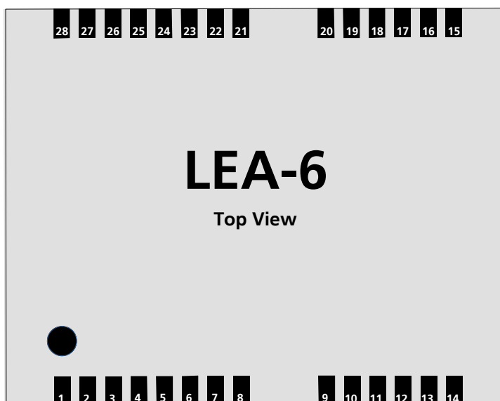
Figure 2 LEA-6 Pin Assignment
