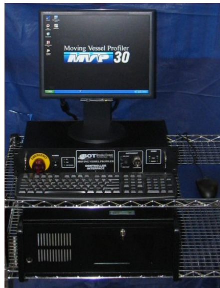
Controller computer and controller interface box
