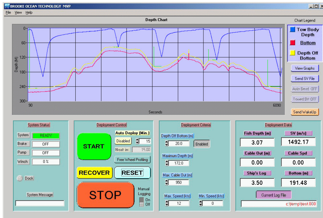
MVP operator interface screen. This will be modified to act as the shore based operator interface for the buoy mounted profiler winch
