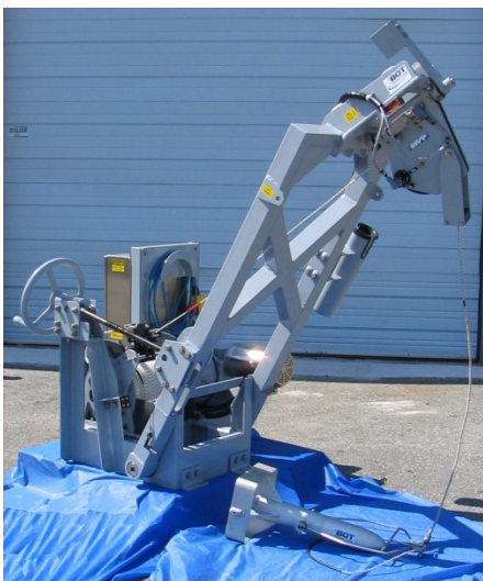
MVP30-350 showing winch and control box. The A-frame is not part of the scope of supply.
