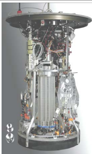
Figure 1. Second generation ESP instrument (16" d x 30" h). bottom left: puck magnified ~2x relative to those loaded in the carousel. See also: http://www.mbari.org/ESP/esp2G_compare.htm
