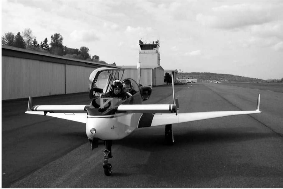
Fig. 1. Photograph of the experimental two-seater, pusher-prop Vari-Viggen aircraft with mounted SPR sensor, its pilot and its sensor operator.
