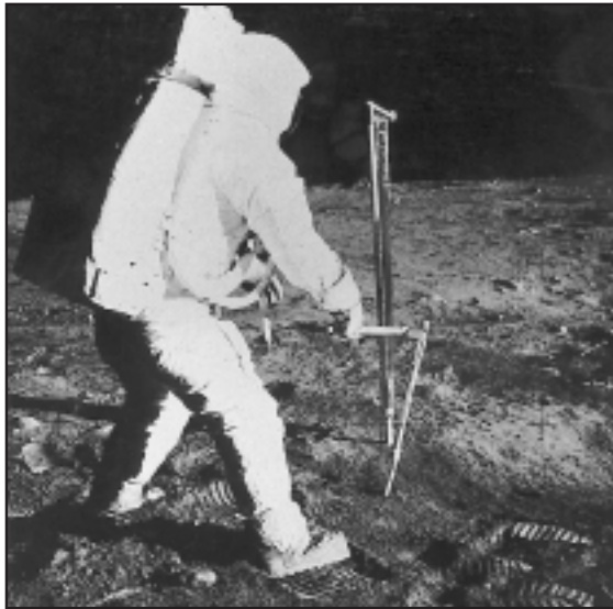
CANADIZE treatment on both the inside and outside of the titanium core-sample drill tubes used in NASA's exploration of the moon's surface prevented galling at the joints and in the drive shaft. It also eliminated the danger of contamination of moon rocks samples by titanium particles or other foreign materials.
