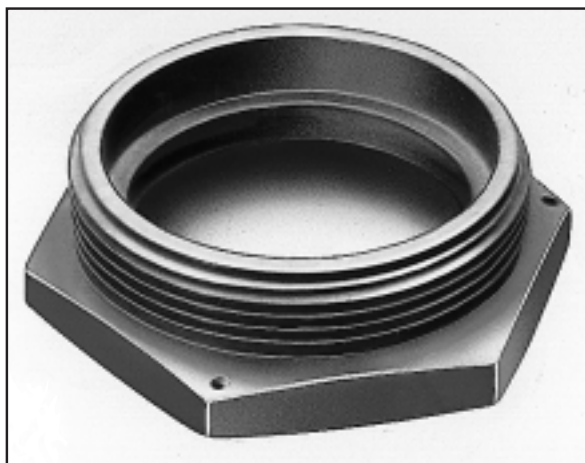
Titanium gland nuts used in aircraft are protected against freeze-up, abrasive wear and corrosion by a CANADIZE surface treatment. The dry-lubrication of the coating also permits faster maintenance procedures.
