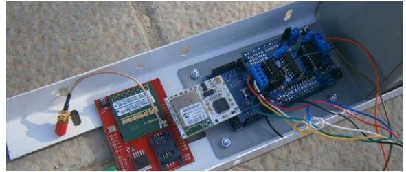
Fig. 19. Basic electronic modules placed on watertight internal structure
