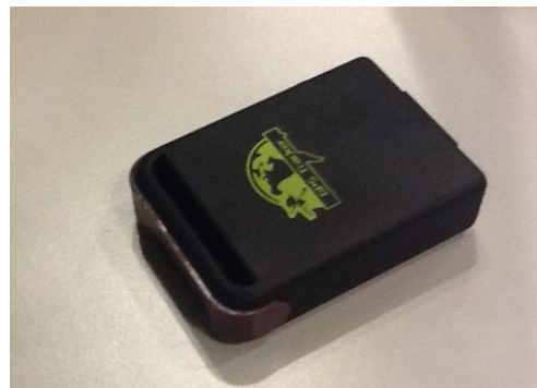
Fig. 20. GPS UMTS tracker with 48 hours of autonomy
