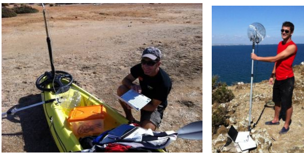
Fig. 21. GPS UMTS tracker and WiFi test carried out during this year in the mar Menor area and inner islands.
