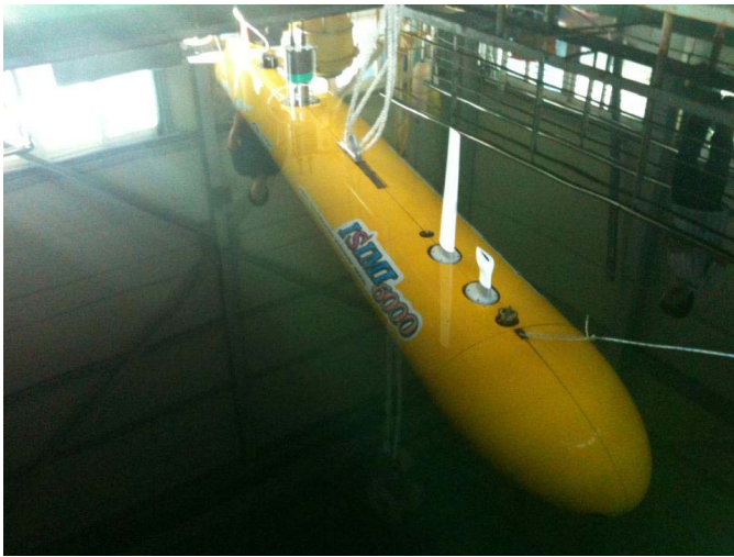
Fig. 1. Ballasting appearance of the ISiMI6000 AUV.
