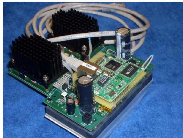
Fig. 5. The pill power supply showing its unique shape
