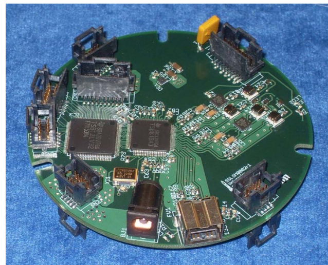
Fig. 14. Top of the communications board
