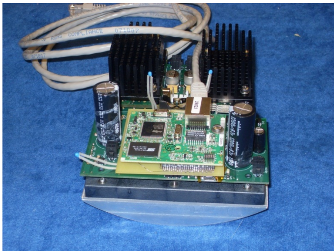
Fig. 4. The pill power supply
