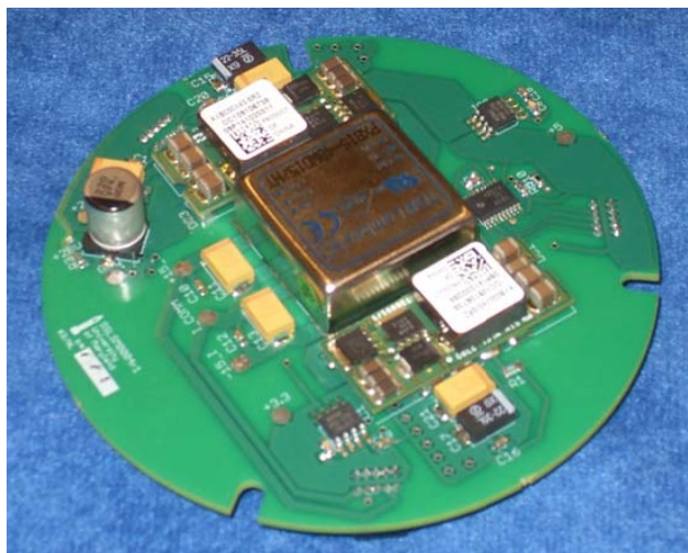
Fig. 11. The DC/DC conversion board
