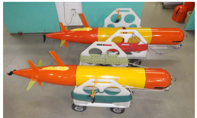
Figure 1: Two Tethys-class Long Range AUVs: Tethys in foreground and Daphne with a long-nose configuration in back.
