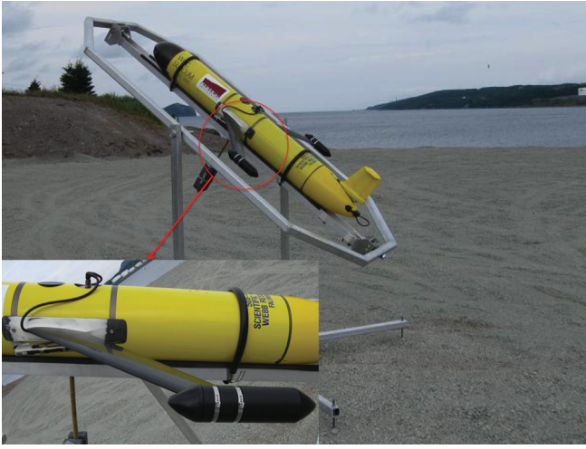
Fig. 10. Hybrid glider setup for sensor calibration. Fluxgate magnetometers are installed on each of the wing-tips of the glider.
