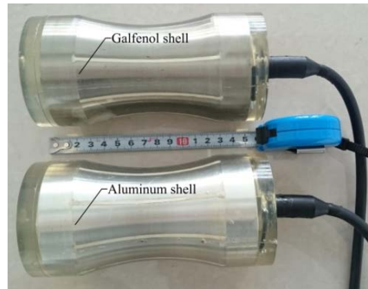
FIG. 10. The prototype barrel-stave transducers with Galfenol shell and aluminum shell.
