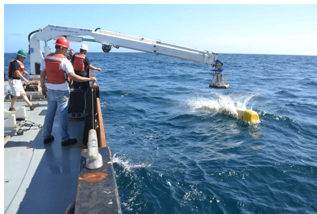
Fig. 1. AUV Launch from RV Rachel Carson
