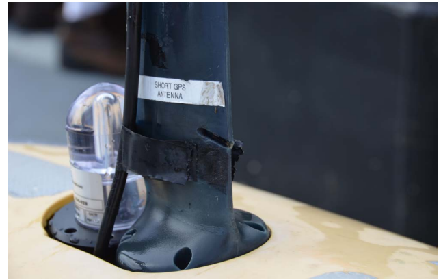
Fig. 12. AUV Antenna damage
