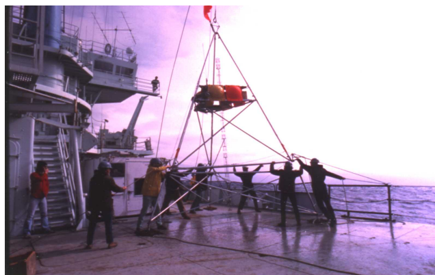
Fig. 5. The insertion of a recovered (floated to the surface) BASS array of sensors required careful alignment with the next expendable tripod base. The release system was justified by the need to get simultaneous data from as many as four of these BASS tripods over a period of half a year at the HEBBLE site on the lower slope off New England.
