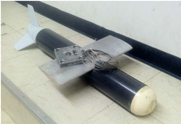
Figure 2. Picture of testing model the 3.4m cable and plate used to attach to the force gages.
