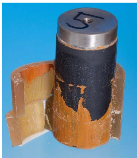
Fig. 14. EY5 NCC coated cylindrical sample after circumferential peel testing. The top-most peel band has completely deboned from the NCC coating, and the middle peel band is well on its way to suffering a similar fate. The lower-most peel band is still well bonded and exhibited polyurethane cohesive failure.
