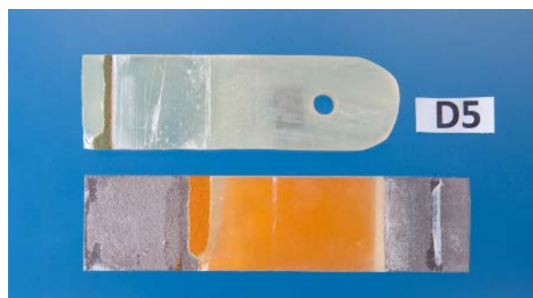
Figure 9: DGO-1 coated flat bar ALT sample after peel testing. This sample was overmolded with PR-420 primer and PR-1547 polyurethane and had spent one week in the 66°C ALT under cathodic delamination conditions before it was peel tested. The greenish material attached to the right side of the PR-1547 is DGO-1 that has debonded from the metal coupon in a quasi-“window-frame” like pattern.
