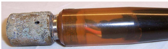
Fig. 15. Outboard cable connector suffering from cathodic delamination. The dark region on the backshell under the polyurethane overmold has already debonded; only the orange portion of the backshell is still bonded. Note that the debonding has proceeded inward from the exposed metal/coating edge.
