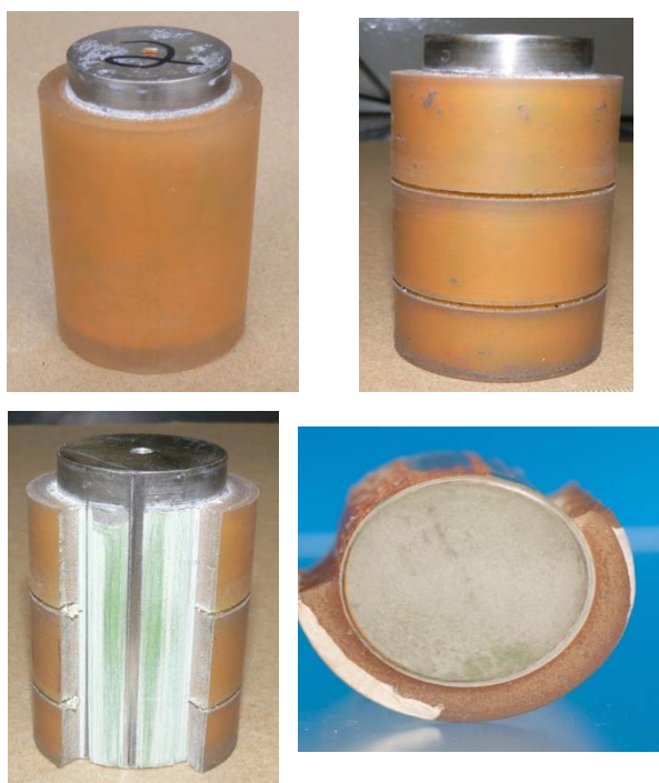
Fig. 7. Preparation of a cylindrical sample for peel testing. First row, left to right: the zinc anode is removed and the sample is cleaned prior to machining; two parallel cuts are made through the polyurethane to the DGO-1 layer. Second row, left to right: a 1.0 inch (2.54 cm) wide cut is made down the side of the cylinder, removing the polyurethane down to the DGO-1 layer; and the bottom 0.25 inch (6.4 cm) portion of the polyurethane layer is removed.
