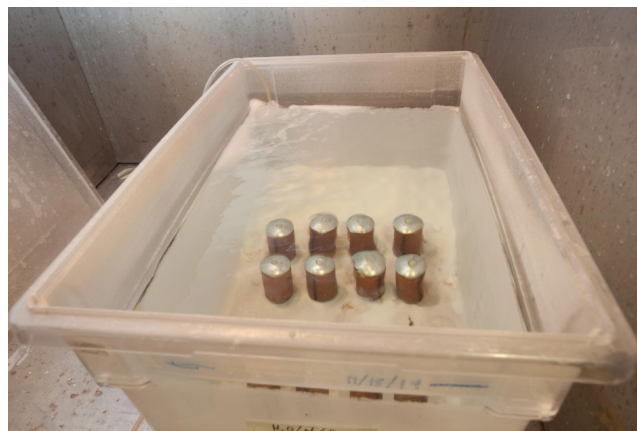
Fig. 8. The ALT tank being bubbled with oxygen gas (back left corner). Eight cylindrical samples are in the tank.
