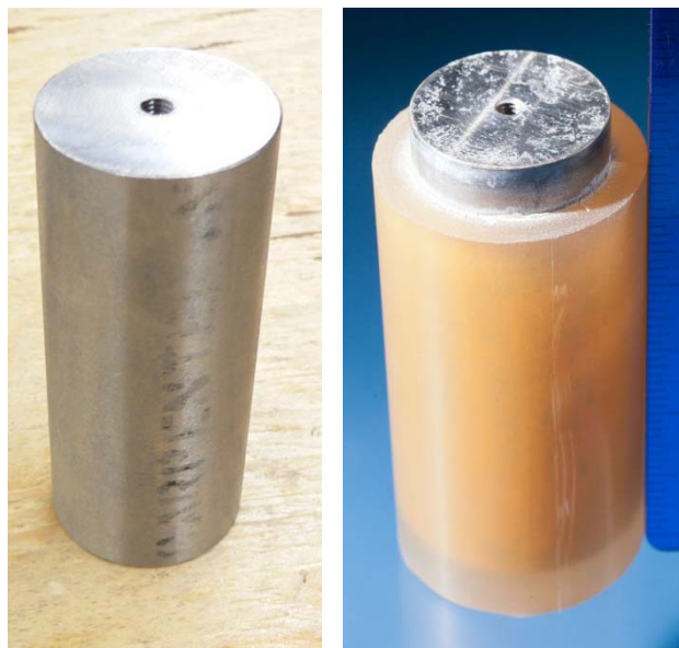
Fig. 4. Uncoated and coated cylindrical “round-stock” samples. Note that the coated sample is uniformly overmolded with a 0.25 inch (6.4 cm) thick layer of polyurethane except for the last 0.25 inches (6.4 cm) of the top end of the cylinder.
