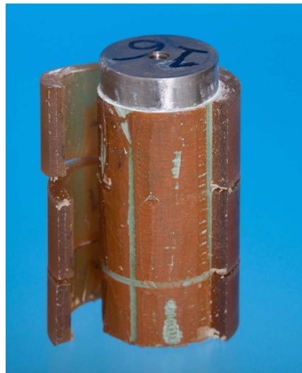
Fig. 11. EY16 cylindrical sample with DGO-1 coating after circumferential peel testing. Each of the three polyurethane peel strips failed cohesively.
