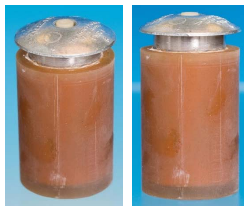
Fig. 6. Completely molded cylindrical samples with sacrificial zinc anodes attached. These samples are ready to be placed into the ALT tank.
