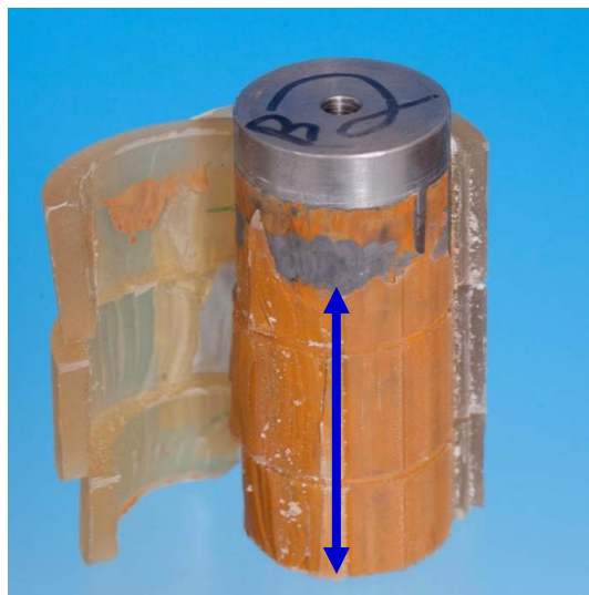
Fig. 13. EY2 bare metal cylindrical sample after circumferential peel testing. The blue arrow indicates the extent of the still well-bonded region.
