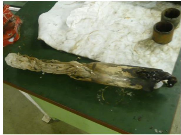
Fig. 10 Melted Core Liner (0.7 m, originally 9.5 m) in Exp.331
