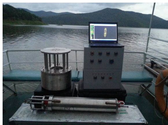
Fig. 1. Components of the LBL system tested in the field trial, including transducer, transponder, computer, signal processing box and power box (counter-clockwise from top left).
