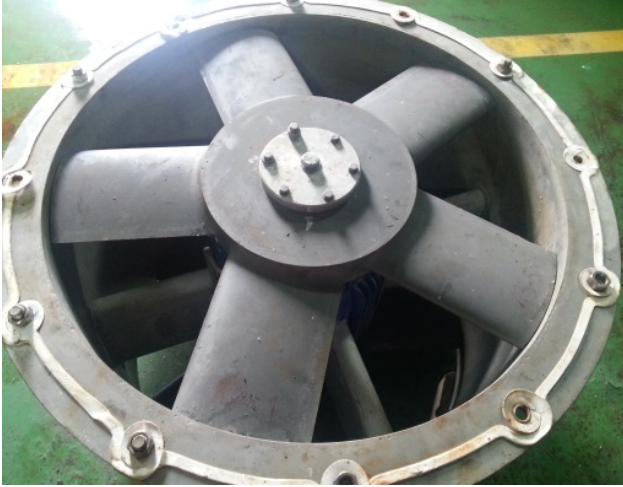
Fig.2. Wells turbine in Mutriku wave plant
