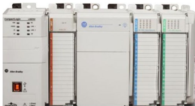
Fig. 3. An Allen-Bradley CompactLogix PLC with 3 I/O cards. From left to right; a L36-ERM processor; 1769-IF16V 16 analog input module; 1769-PA4 4-amp power supply; 1769-IG16 16 input TTL module; 1769-OV16 16 output 24V DC sinking module.
