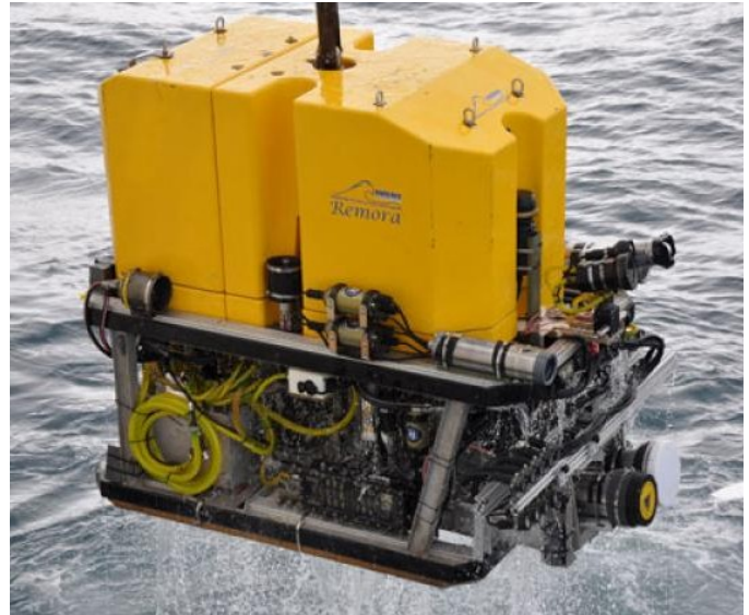
Fig. 1. Remora III Remotely Operated Vehicle being recovered after an operation.
