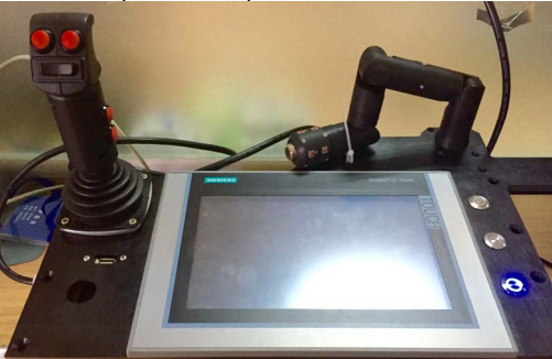
Fig. 5 Control box. It's a multifunctional control box, in the left the handle with red buttons is used to control a 5 functional manipulator, the right handle is used to control the 7 functional manipulator.
