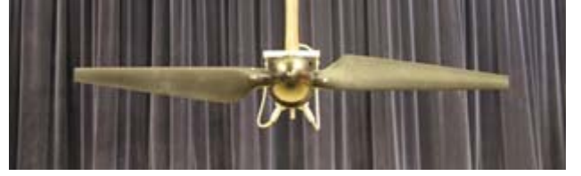
Fig. 2: The two-bladed horizontal axis marine current turbine used in the present experiment, shown mounted to the dynamometer with the data acquisition cables for thrust and torque protruding from below.
