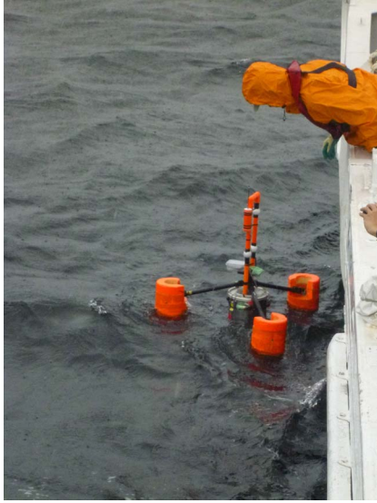
Fig. 5. Ultra-small-buoy for wave measurement developed by Yokohama National University
