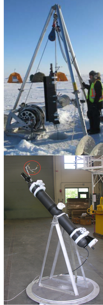
Fig. 2. a) ITP-V (ITP 78) during deployment through a hole in the ice. b) ITP-V profiler in the jig for pre-deployment spin tests. The MAVS is circled in red. Spin tests were performed outside on a pad designed to be free of magnetic anomalies.
