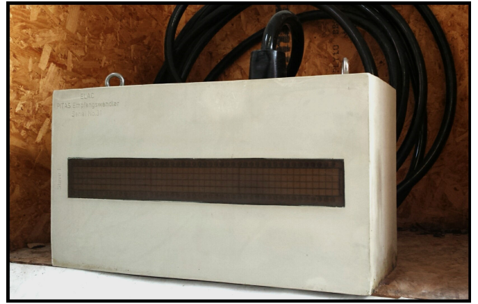
Figure 1. Receiver hardware for the proposed sonar signal processing. The receiver consists of 48 channels. The transmitter (not depicted) consists of 32 channels.
