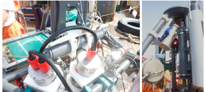
Fig. 2. Niskin bottle equipped for bottom water sampling (left) and for specified depth water sampling (right).
