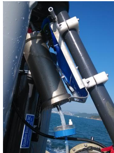
Fig. 3. In-situ microorganisms enriching and fixation device.
