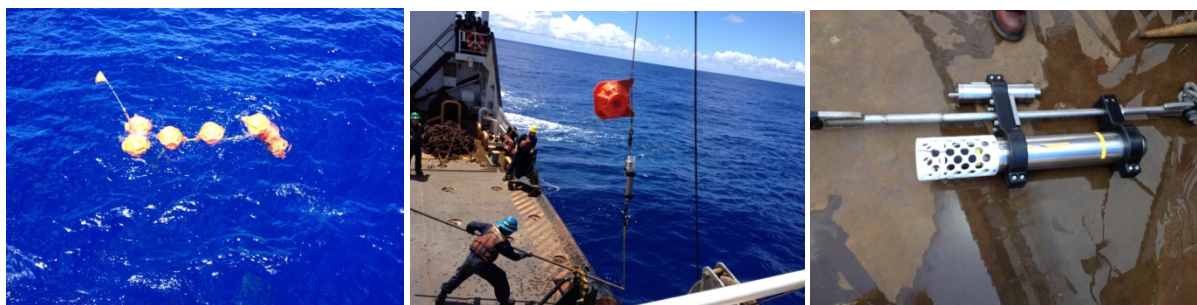
Fig 5: Left image shows floats and mast once the mooring made it to the sea surface. Middle image shows recovery of sensors and float onto ship. Right image shows close up of hydrophone and pressure sensor immediately after recovery.
