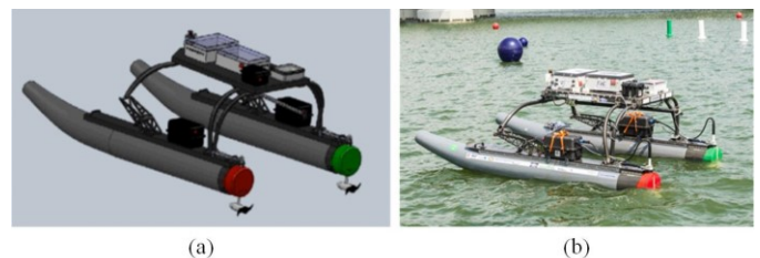
Fig. 1. View of the actuators on the USV16 model (a). The USV16 vehicle in transit during the RobotX Maritime Challenge in Marina Bay, Singapore (b).
